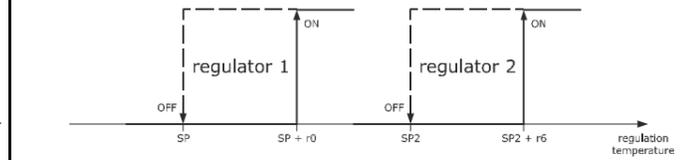
Cold mode regulation setpoint 1 (r5 = 0) and hot mode regulation setpoint 2 (r10 = 1).
