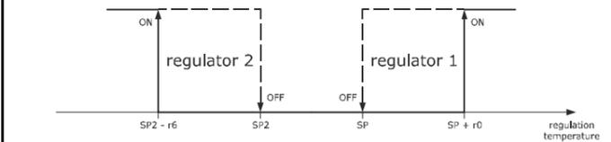
Hot mode regulation setpoint 1 (r5 = 1) and cold mode regulation setpoint 2 (r10 = 0).
