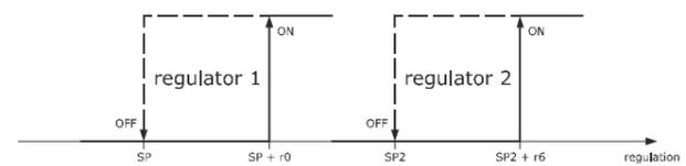
Cold mode regulation setpoint 1 (r5 = 0) and hot mode regulation setpoint 2 (r10 = 1).
