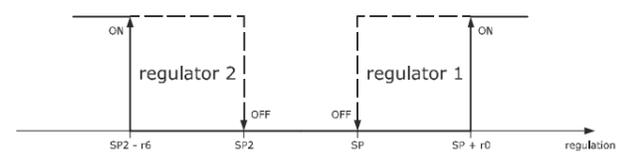
Hot mode regulation setpoint 1 (r5 = 1) and cold mode regulation setpoint 2 (r10 = 0).
