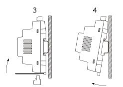
To install the devices again press the DIN rail clips to the end
