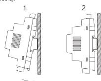
To remove the devices remove possible extractable screw terminal blocks plugged at the bottom first, then operate on the DIN rail clips with a screwdriver as shown in the following drawing.
