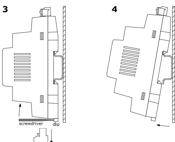
To install the device again press down the clip before.
