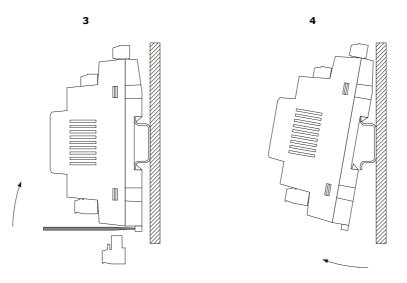
To install the devices again, first press the clip of the DIN track.
