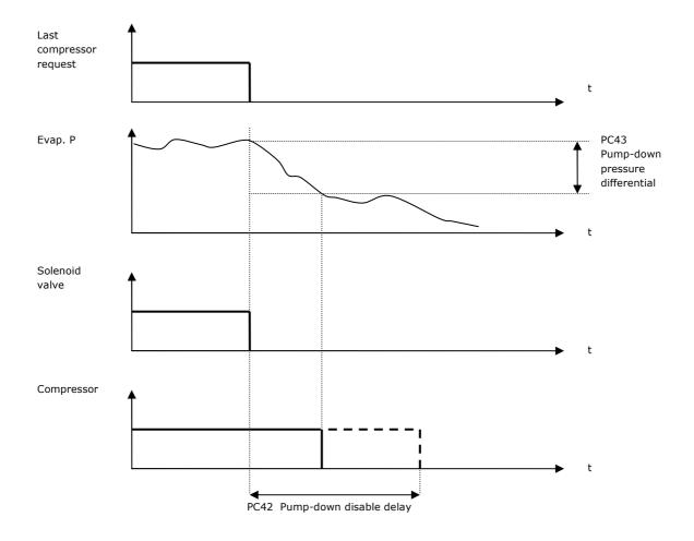
Anyway, there is always the Compressor switch-OFF delay in pump-down, should the switch-OFF pressure threshold not be reached, or should evaporation sensors be faulty.
