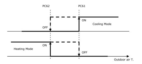
WARNING – Operating mode change-over can also happen while the machine is ON: in this case, the machine switches itself OFF – complying with all its timings – then commutates, and thereafter switches itself back ON automatically.
