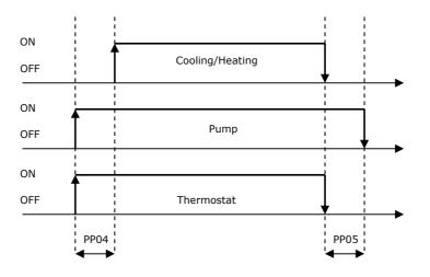
In similar fashion, upon a thermostat's switch-OFF request, the compressor switches OFF, whereas the pump remains ON for the duration of PP05.
