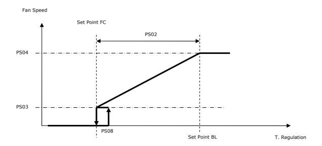
When the temperature reaches the FC Set Point and remains below for more than *PS10* seconds, it deactivates free-cooling; the step shown in the diagram, hysteresis *PS08*(default 0.5°C), re-enables free-cooling and the ramp (if ON status is maintained for more than *PS10* seconds).
