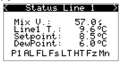
P1: Pump discharge line on
