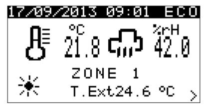
Main screen that displays date, time, time slot current, temperature, humidity, outside temperature, season and zone name. Press RIGHT to access the configuration screen area.
