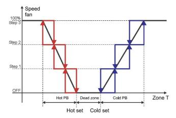
For the ventilation 3 step activation will be divided the proportional band in equal parts (will be the same of the zone valve).
