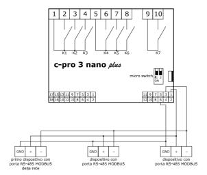
In the example, the c-pro 3 nano plus is the last device on the network with an RS-485 MODBUS port.
