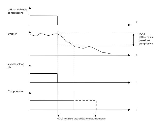
In the event that the switch-off pressure threshold is not reached or if the evaporation probes don't work, there is always a Compressor switch-off delay in pump-down.
