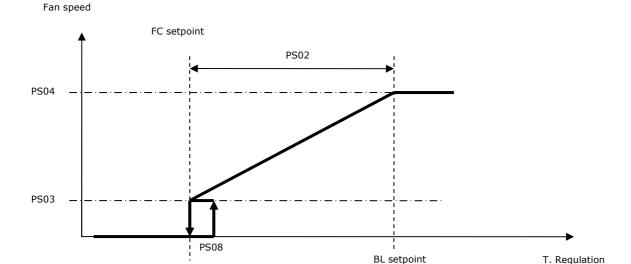
When the temperature reaches the FC setpoint and stays below it for more than *PS10* seconds, the free-cooling is deactivated; the step indicated in the diagram, of hysteresis PS08 (default 0.5°C), re-enables the free-cooling and the ramp (if the ON mode is maintained for more than *PS10* seconds).
