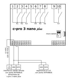
The maximum configuration of the INTRABUS network permits 1 programmable controller and 1 remote repeater.
