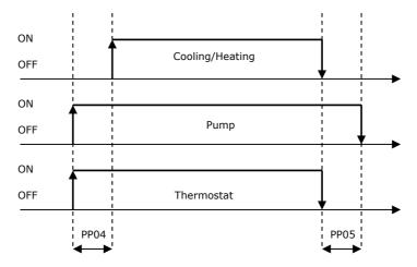
Similarly, following a thermostat switch-off request, the compressor switches off, while the pump stays on for the duration of PP05. In the *cyclical operation, the* pump is controlled by the definition of the start-up/switch-off times: if during pump activation time the thermostat function activates a cooling or heating request, the pump stays active for the entire duration of this request, plus any delay interval between compressor switch-off and pump switch-off.
