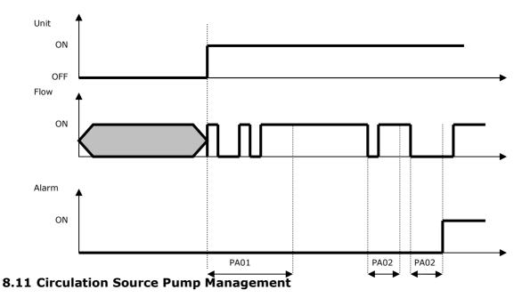
On the WATER/WATER machines you can control one or two water circulation source pumps, which are set in parameter *PG10*. The *Pump operation PP21* parameter sets how the pump will work.
