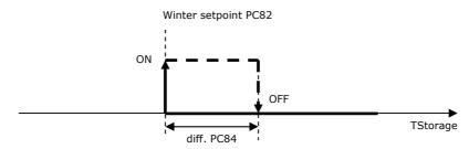
To use this function you need to enable the auxiliary regulation probe in the *HAxx* parameters.
