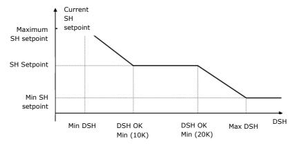
This way the risk of liquid return to the compressor is limited and system efficiency increases based on the machine's working conditions.
