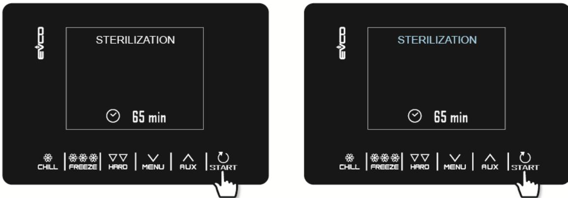
Sterilisation ends when the time set by parameter u6 has elapsed, after the **START** key has been pressed for 2 seconds or if the door is opened. During sterilisation the cabinet sterilisation relay is active. If parameter u11 is set to 1, the evaporator fans are also active.
