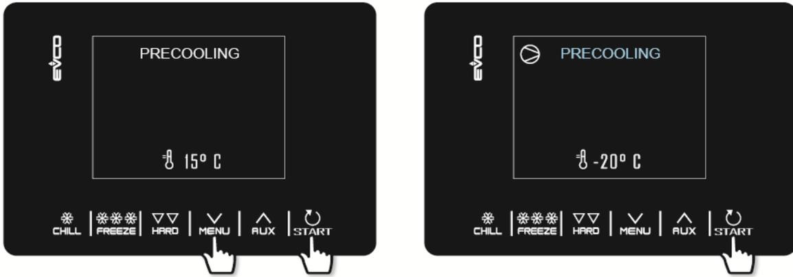
Once the required cabinet setpoint has been reached, the buzzer sounds and the cycle continues and maintains the cabinet temperature achieved until the **START** key is pressed for 2 seconds or until a blast chilling/blast freezing cycle starts up.
