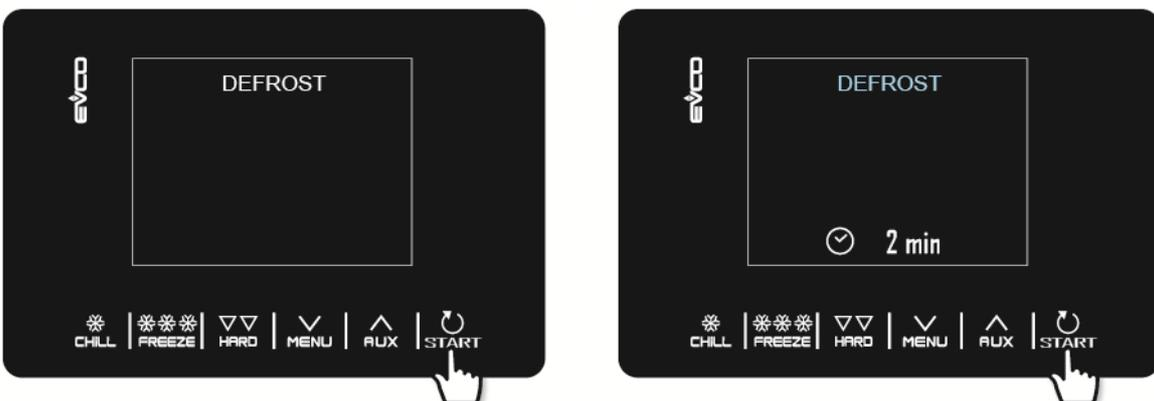
Defrosting can also be carried out automatically during conservation or pre-cooling at time intervals set by parameter d0, provided that this value is not set to 0.
