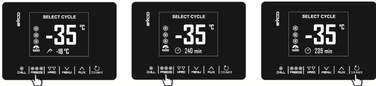
Example of a temperature controlled blast freezing cycle (needle), conversion to time controlled cycle, quick change of the blast freezing cycle duration and start cycle.
