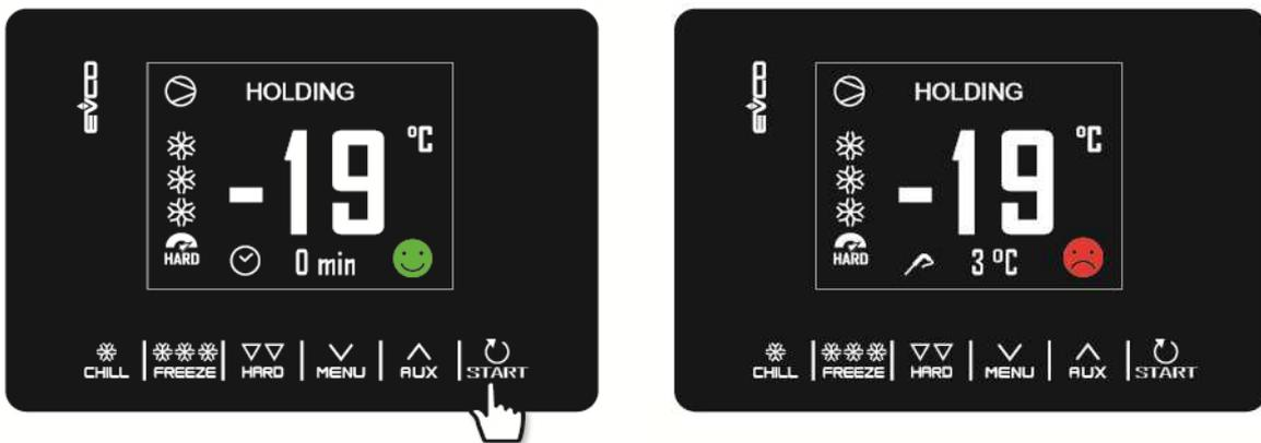
The conservation phase is not timed and is only terminated when the **START** key is pressed for 2 seconds.
