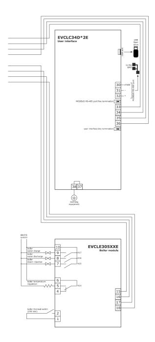
Fan management in "on/off" mode at single speed (parameter F0 = 0).
