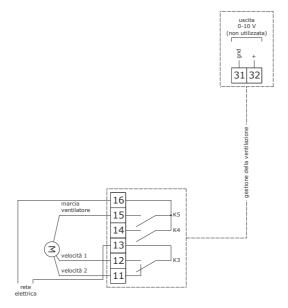
Fan management in modulating mode (parameter F0 = 3).
