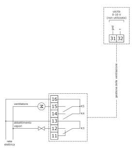
Fan management in "on/off" mode at two-speed (parameter F0 = 2).
