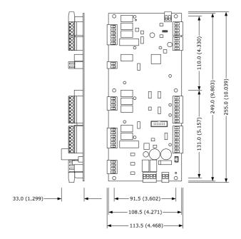
Installation is on a flat surface with spacers.
