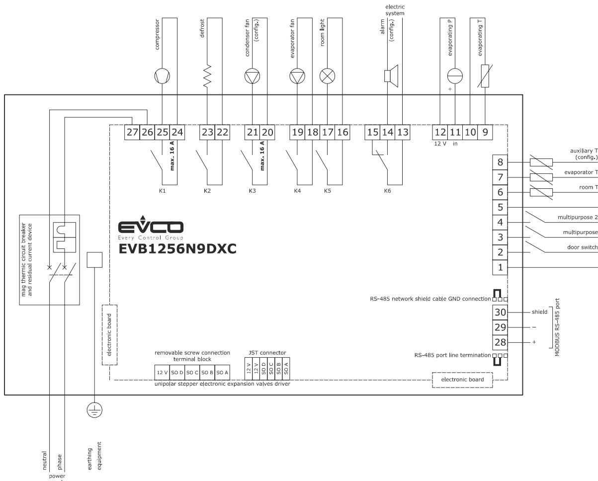
Electrical connection for models with data logging for EN 12830 standard compliance (for example EVB1214N9XLC).
