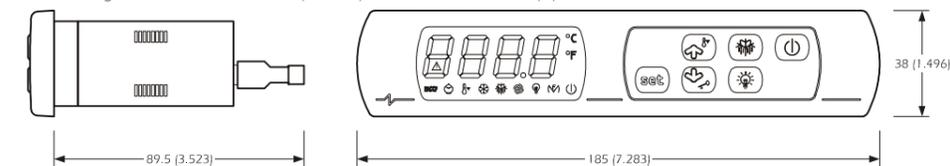
Independently on the kind of connections, the maximum depth is 89.5 mm (3.523 in) and refers to the models with faston (with straight female faston properly plugged).
