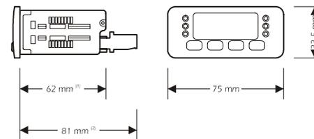
(1) maximum depth with screw terminal blocks (standard model)
