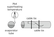
The speed with which the temperature is transmitted determines the accuracy of the instant superheating calculation. Apply a conductive paste and place the sensor with its tip pointing upwards slightly and the
