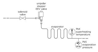
**Pb5**: 4...20mA evaporation pressure transducer. Reading scale from parameters P9 and P10. **Pb4**: superheating temperature sensor. The type of temperature sensor is defined by P0, default NTC. The P0 setting applies to both regulation and superheating.
