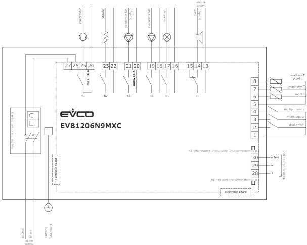
Electrical connection for models with data logging for EN 12830 standard compliance (for example EVB1214N9XLC).
