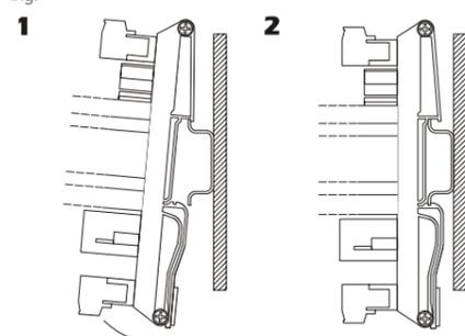
To remove the control module, provide oneself with a screwdriver and operate as shown in the following drawing.
