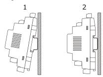
To remove the devices remove possible extractable screw terminal blocks plugged at the bottom first, then operate on the DIN rail clips with a screwdriver as shown in the following
