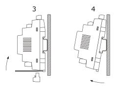
To install the devices again press the DIN rail clips to the end
