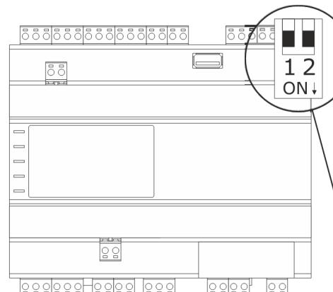
The RS-485 MODBUS network can be polarised using the UNI-PRO 3 development environment.
