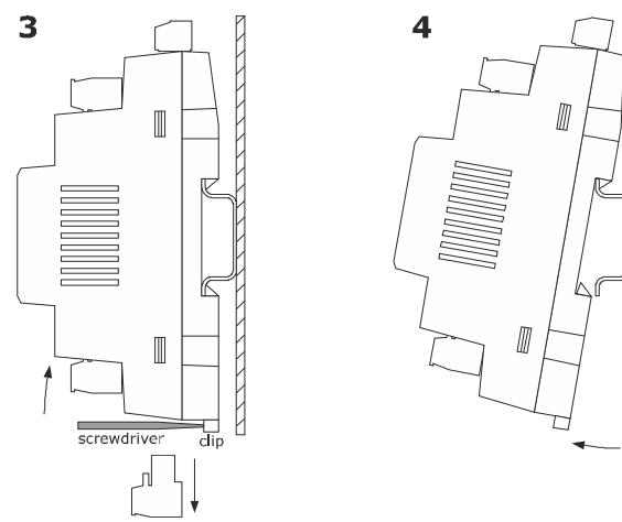
To install the device again press down the clip before.
