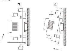
To install EVDRIVE04 again press the DIN rail clips to the end
