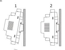
To remove EVDRIVE04 remove possible extractable screw terminal blocks plugged at the bottom first, then operate on the DIN rail clips with a screwdriver as shown in the following drawing
