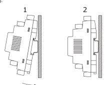
To remove EVDRIVE06 remove possible extractable screw terminal blocks plugged at the bottom first, then operate on the DIN rail clips with a screwdriver as shown in the following drawing
