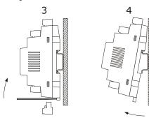
To install EVDRIVE06 again press the DIN rail clips to the end
