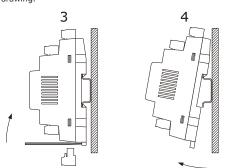
To install EVDRIVE03 again press the DIN rail clips to the end first.
