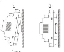
To remove EVDRIVE03 remove possible extractable screw terminal blocks plugged at the bottom first, then operate on the DIN rail clips with a screwdriver as shown in the following
