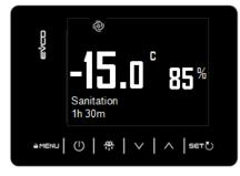
If the  $\boldsymbol{U}\boldsymbol{V}$  function is enabled it will be also displayed on the icons header, the process is performed without stopping the normal temperature and humidity regulation
