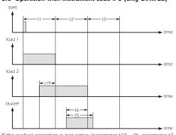
If the cyclical operation is not active (parameter t18 = 0), parameter t3will not be visible
