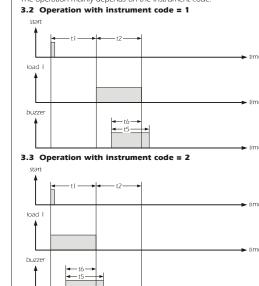
If the cyclical operation is not active (parameter t18 = 0), parameter t2will not be visible
