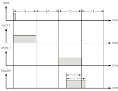
If the cyclical operation is not active (parameter t18 = 0), parameter t4 will not be visible
