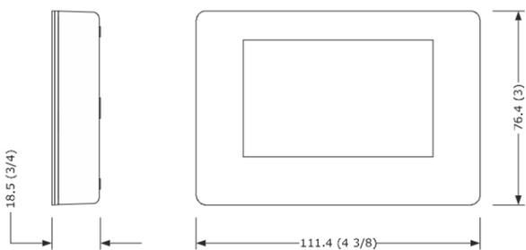
Wall mounting (with bolts and fastening screws) or in the most common flush mounting boxes (with fastening screws).
