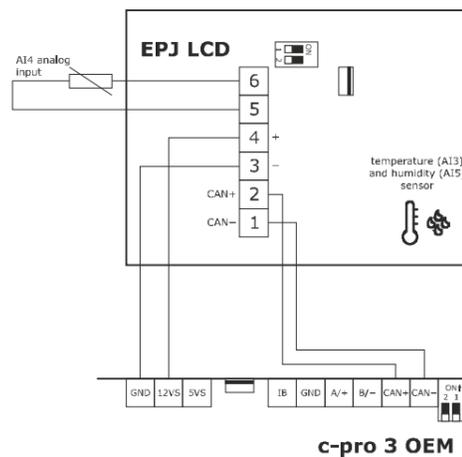
**2.1.4 Pre-setting for the programming and insertion of the CAN port termination resistor**
