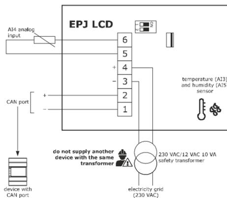
**2.1.3 Electrical connection with device powered by a controller (for example c-pro 3 OEM)**
