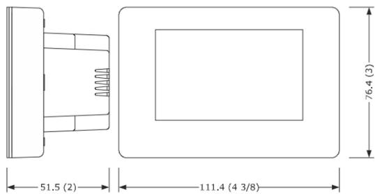
Wall mounting in the most common flush mounting boxes (with fastening screws).
