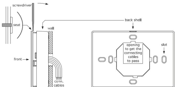
**1.2 Models for wall mounting with back-slot for in-wall box**
