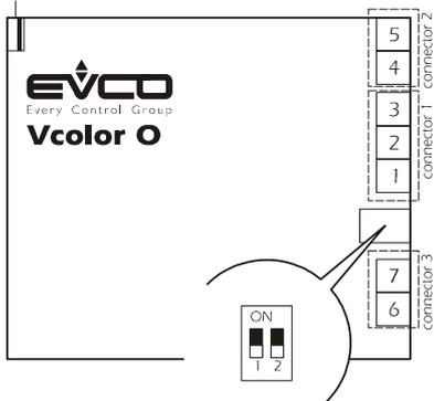
Position micro-switch 1 on position ON to plug in the termination of the RS-485 port; position micro-switch 2 on position ON to plug in the termination of the CAN port.
