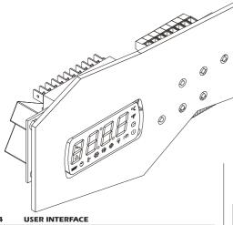
The user interface consists of a custom 4-digit display (with decimal points and function icons) and six keys (SET, UP, DOWN, DEFROST,
