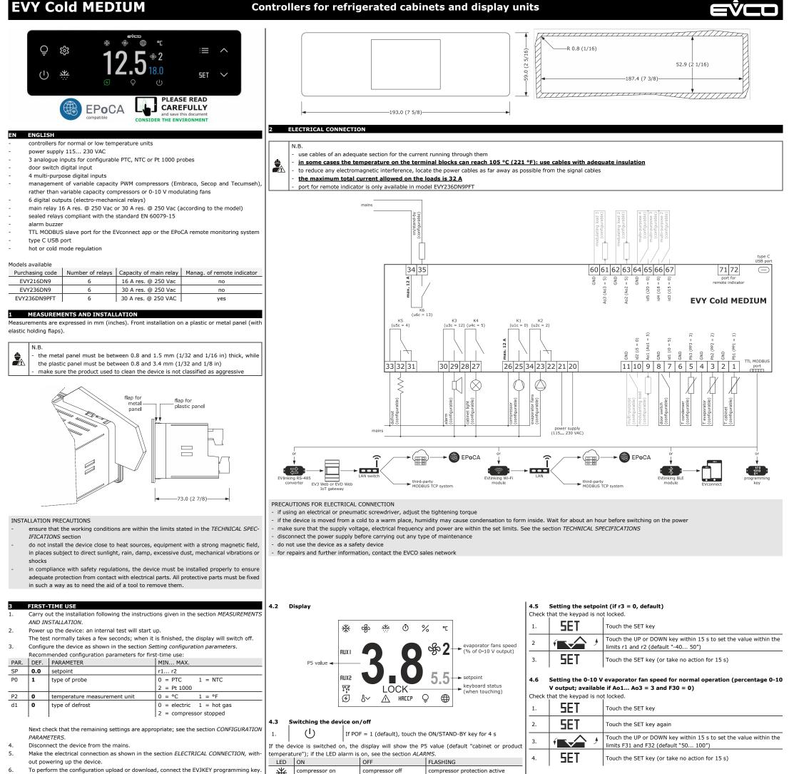
To activate real-time functions, connect the EVlinking RS-485 EVIF23TSX converter. To control the device using the EVconnect app, connect the EVlinking BLE EVIF25TBX module then synchronise it with the app. To control the device using the EPoCA monitoring system or a third-party MODBUS TCP
