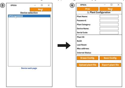
Fig. 23. Selecting the device and configuring the Plant and Device
