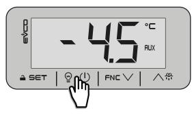
Fig. 13. Activating the AUX output by key
