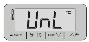
Fig. 10. Confirmation keypad unlocked
