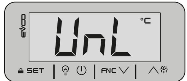
Fig. 10. Confirmation keypad unlocked
