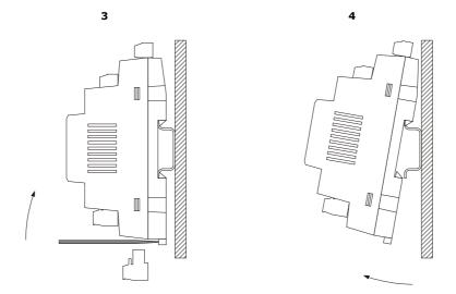
To install the devices again, first press the clip of the DIN track.
