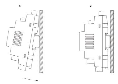
To remove the devices, first remove any screw-in removable terminal boards mounted in the lower part, then trigger the DIN track clip with a screwdriver as show in the following picture:
