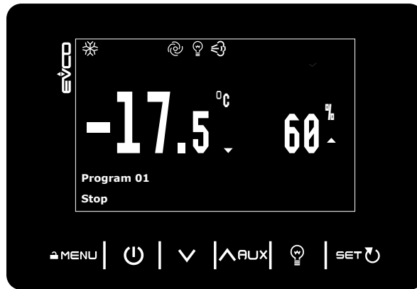
Fig. 11. Display when cycle is stopped
