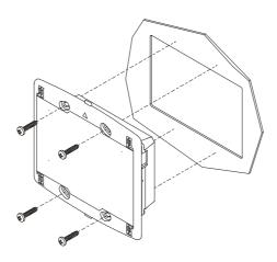
At the front of the sensor one can apply the plates CPVP\* by Evco (to order separately, made in plastic material and available in two different colorations, white and black); look at chapter 6 (ACCESSORIES).
