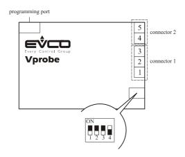
Position micro-switch 4 on position ON to plug in the termination of the CAN port; micro-switches 1, 2 and 3 are reserved. The following tables show the meaning of the connectors.
