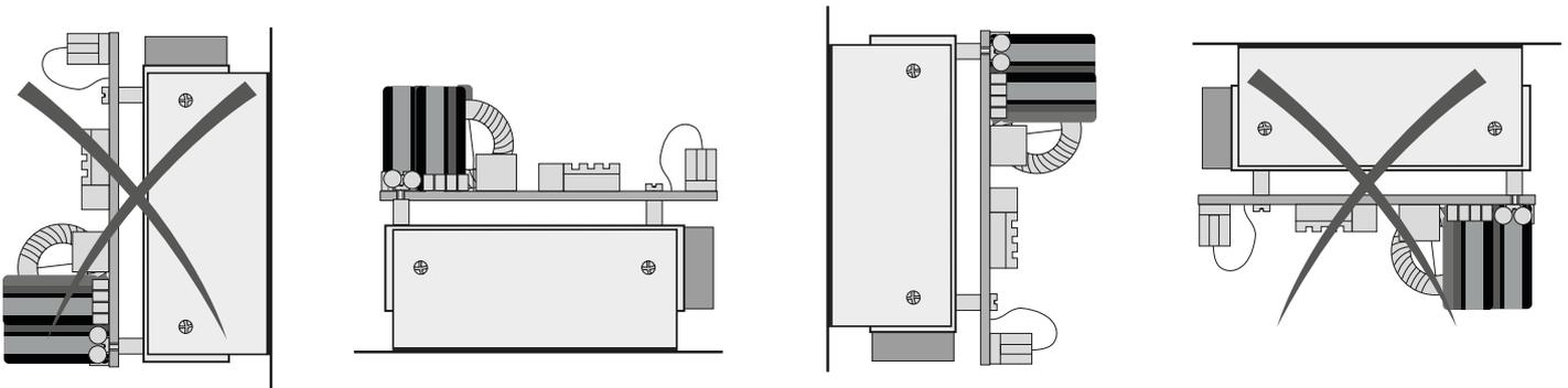
Fig. 1. Inverter installation positioning
