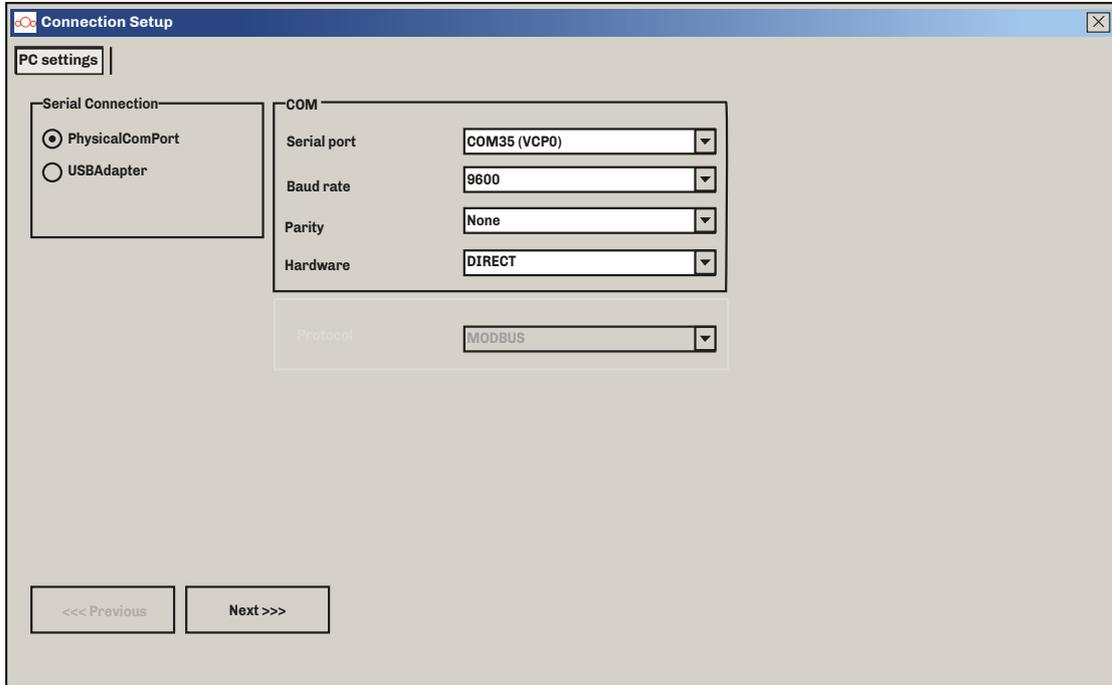
**Fig. 15.** Communication port setting
