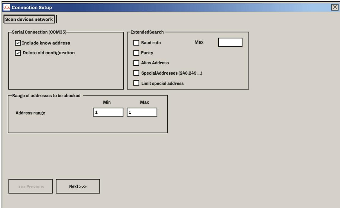
**Fig. 16.** Communication Modbus address setting
