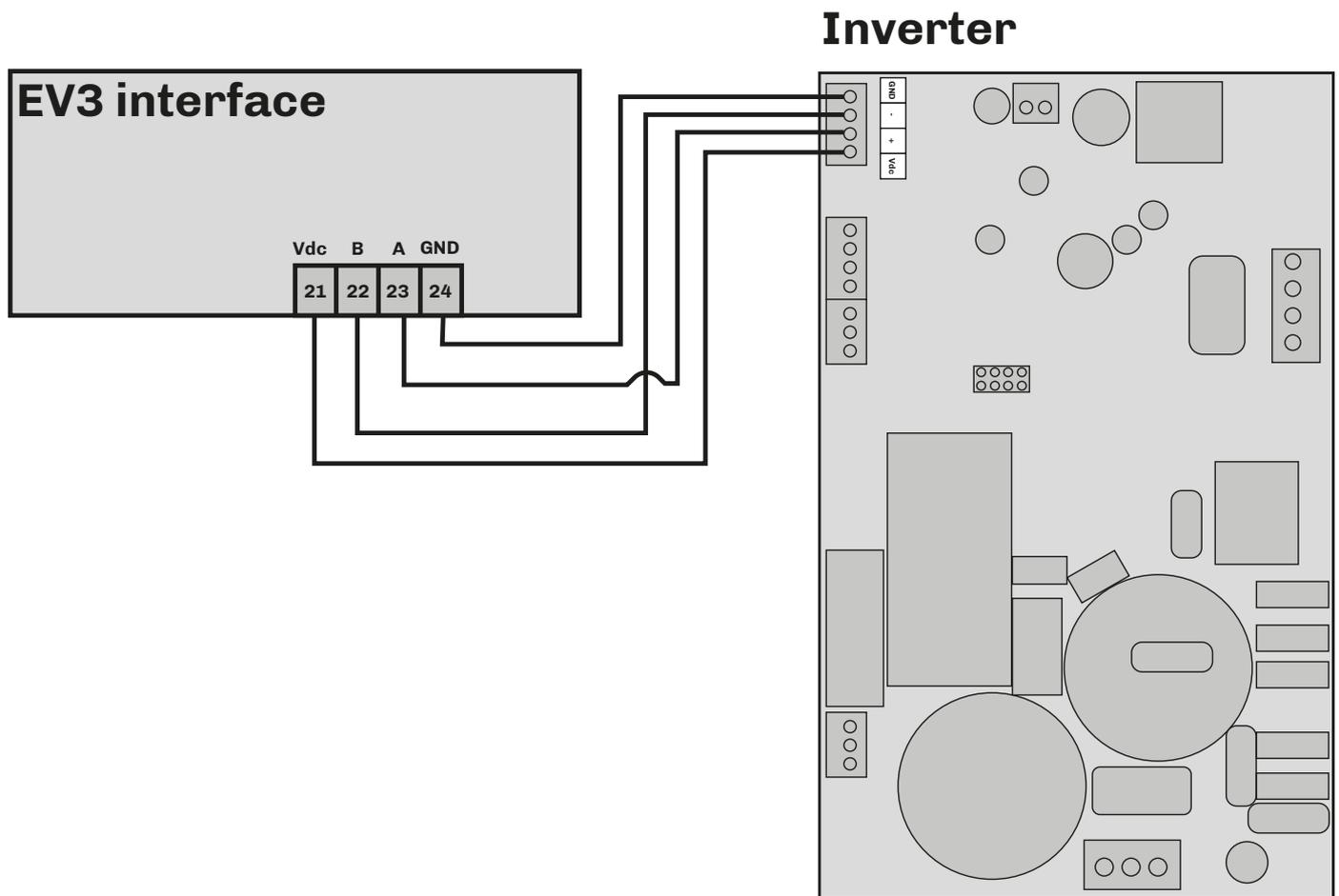
**Fig. 10.** Connection between **Inverter** and **EV3** Interface
