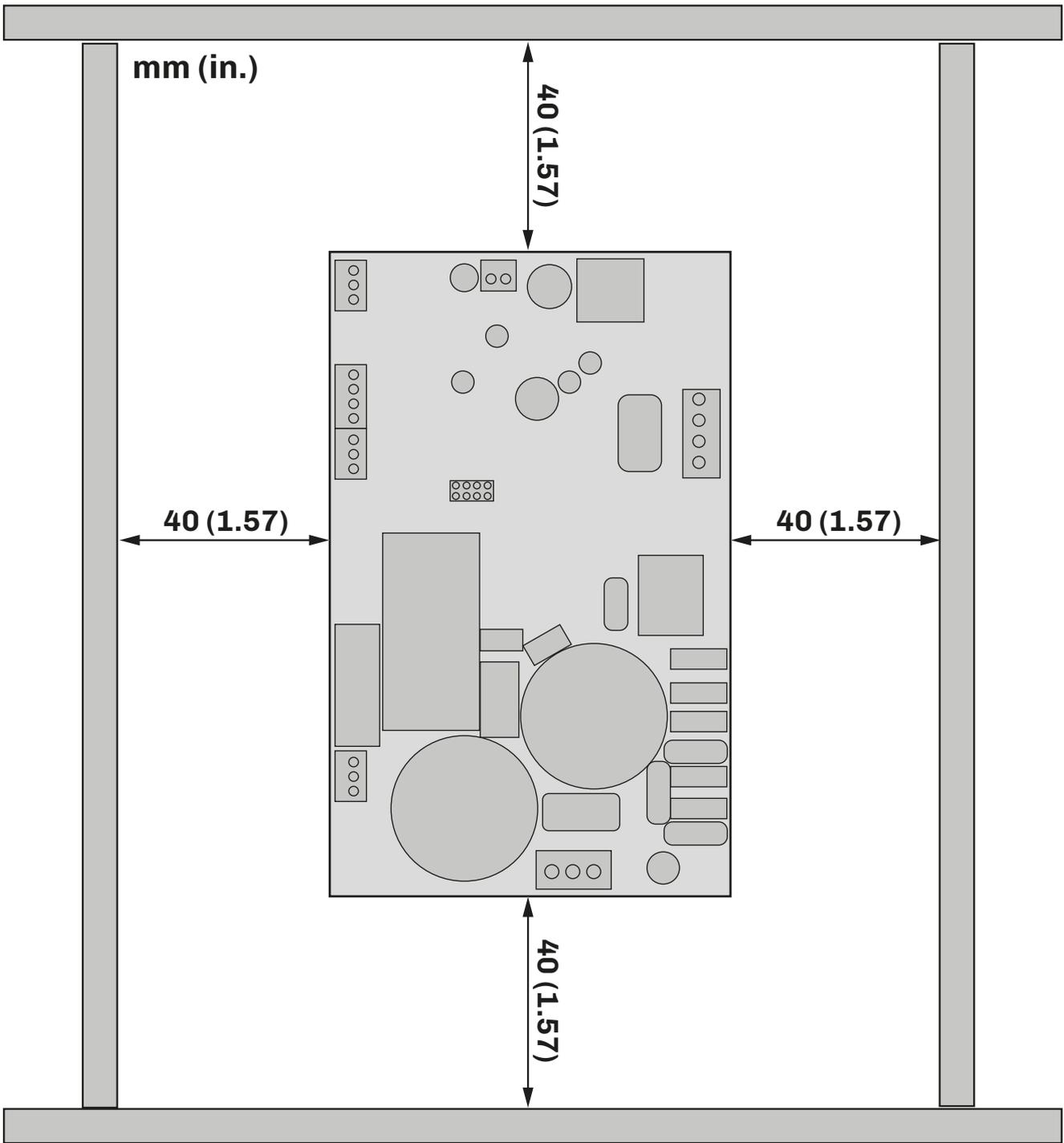
**Fig. 4. Inverter minimum installation distances - view from above**
