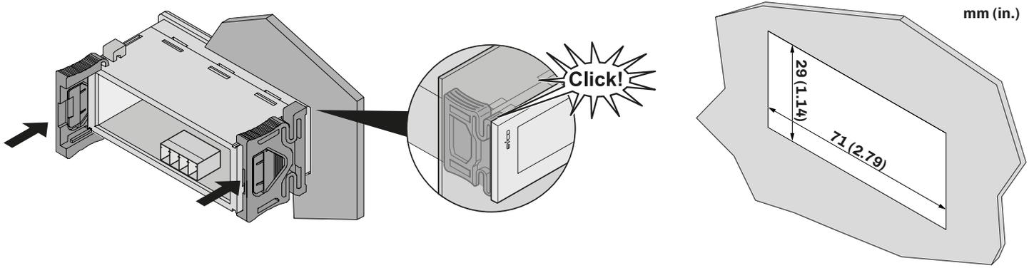
**Fig. 5.** Installing EV3 interfaces
