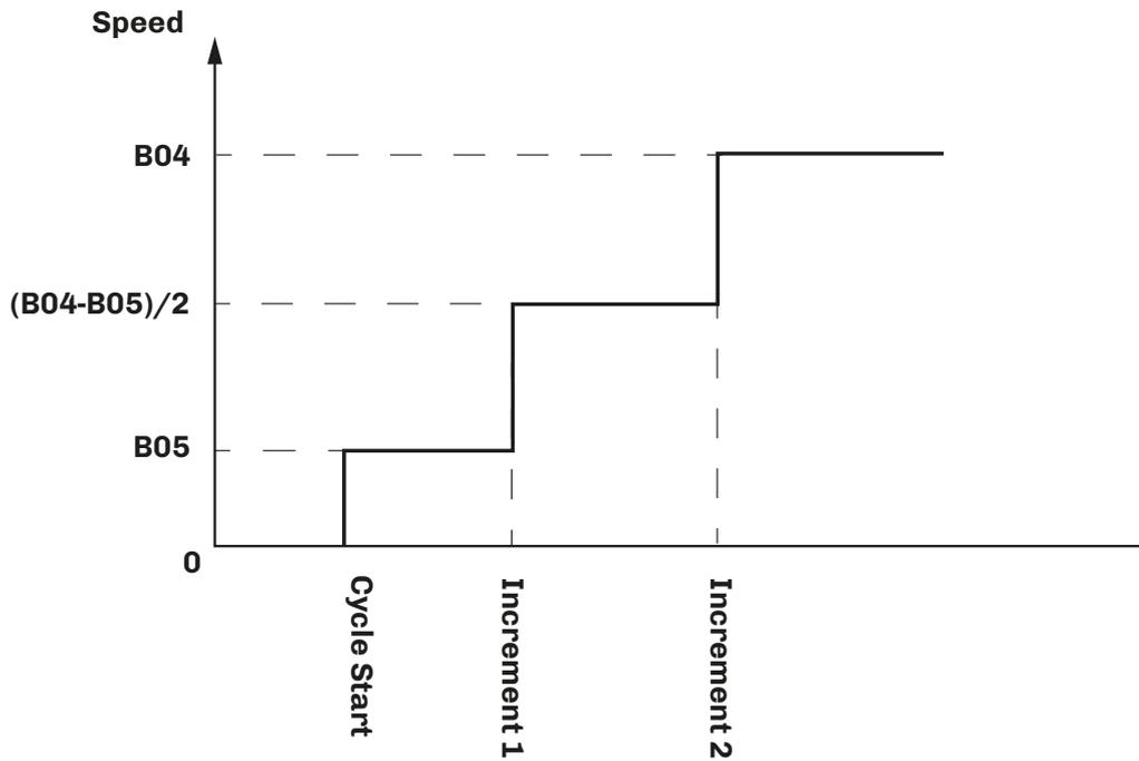
Fig. 13. Setting the speed - Basic interface
