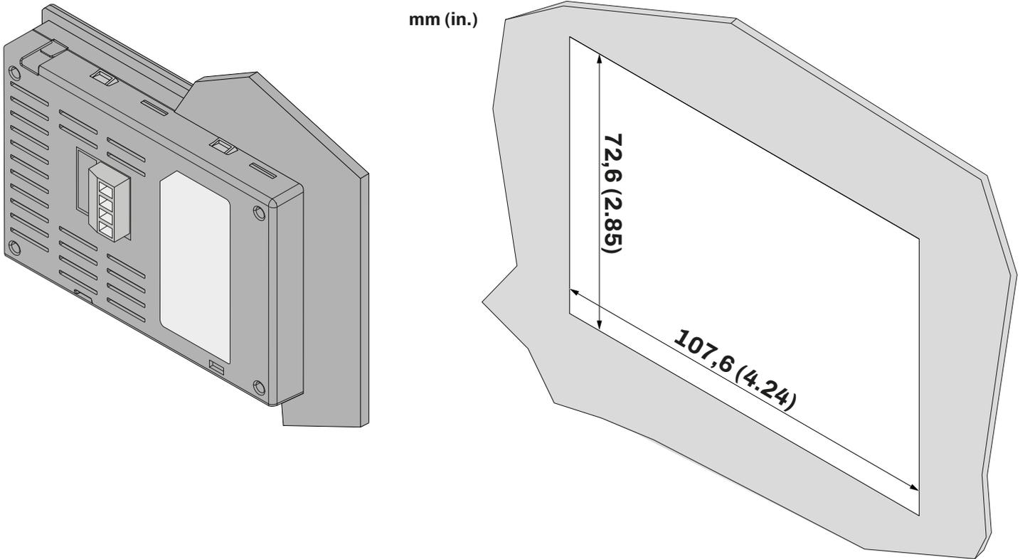
Fig. 7. Installing EVJ interfaces
