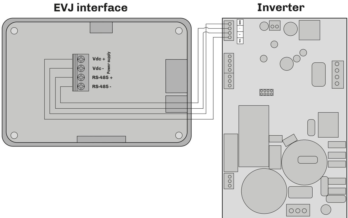
**Fig. 11.** Connection between **Inverter** and **EVJ** Interface
