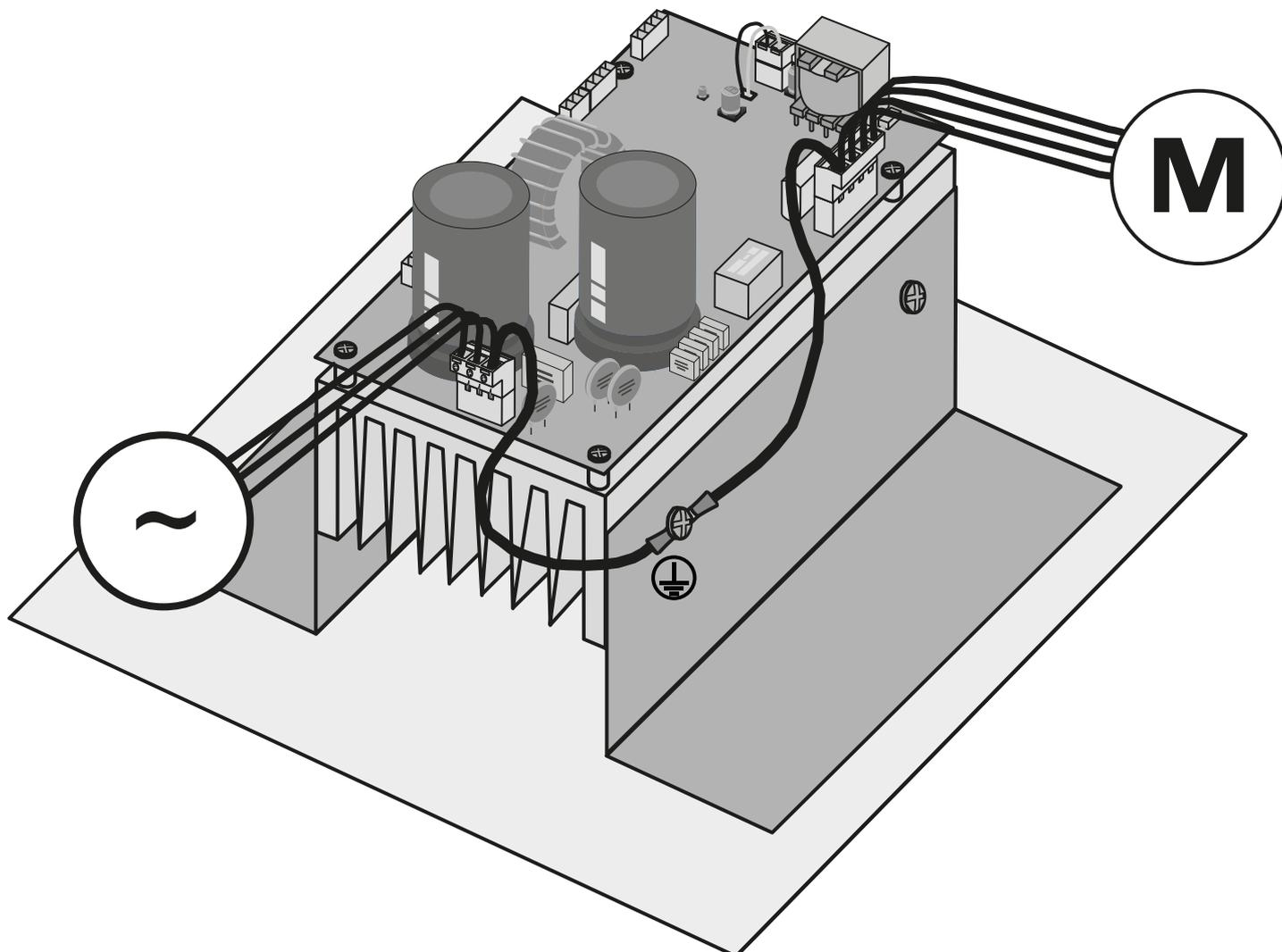
**Fig. 9.** Inverter earthing
