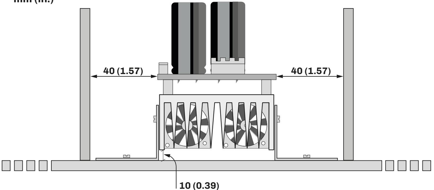
Fig. 3. Inverter minimum installation distances - front view
