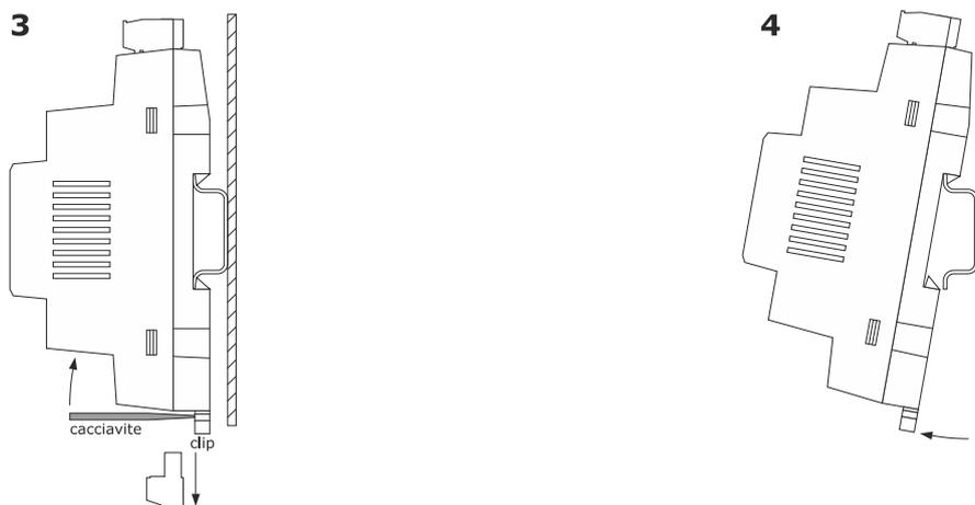
Before re-installing the device, press the clip fully in.
