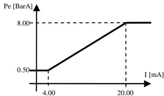
Each of the analog inputs may be configured as "scaling" (Piax = 30), this means its settings will be determined by parameters:
