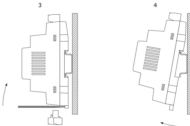
To install the device again press the DIN rail clips to the end first.
