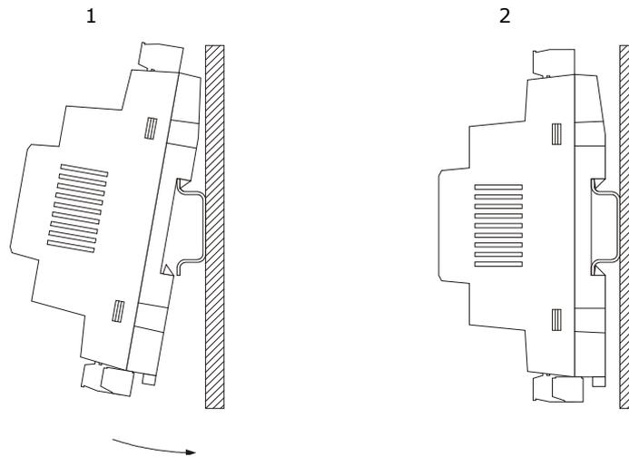
To remove the device remove possible extractable screw terminal blocks plugged at the bottom first, then operate on the DIN rail clips with a screwdriver as shown in the following drawing.
