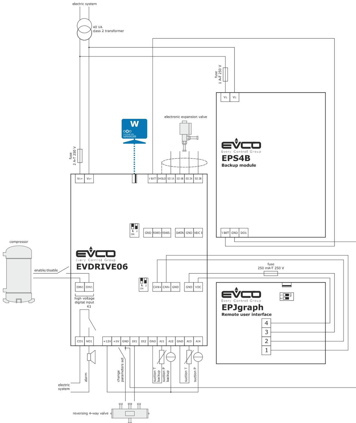
**Please note the power supply of EVDRIVE06 and that of EPS4B are not isolated one another: it is important to wire correctly the devices as indicated in the drawing.**
