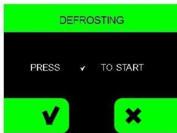
Note : if parameter S01 is not properly configured, no defrosting cycle is allowed when pressing this key.
