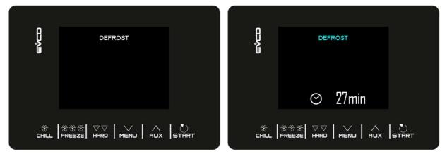
Defrosting can also be carried out automatically <u>during conservation or pre-cooling</u> at time intervals set by parameter d0, provided that this value is not set to 0.
