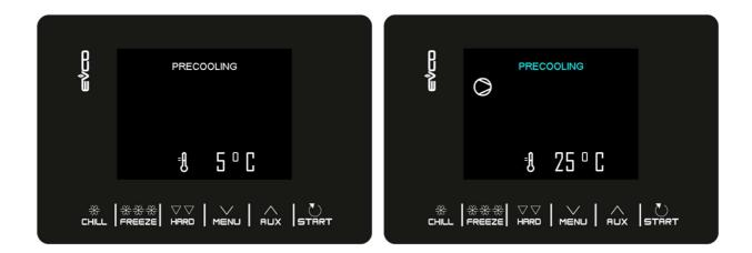
Once the required cabinet setpoint has been reached, the buzzer sounds and the cycle continues and maintains the
