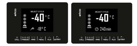
If it is a temperature controlled cycle, a test will be performed to check that the needle probe has been correctly inserted in the food item to be blast chilled. If the test is not successful, the cycle automatically switches to time controlled mode: the buzzer sounds and the type of cycle control is converted from temperature to time on the display. For more details about how to run the test, see section 6.2.
