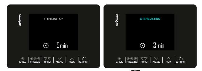
Sterilisation ends when the time set by parameter u6 has elapsed, after the **ETRET** key has been pressed for 2 seconds or if the door is opened.
