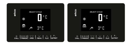
The selected cycle will offer either the pre-loaded settings for that cycle, or the settings of the last cycle carried out (depending on the r36 parameter). By pressing with the permitted ranges.
