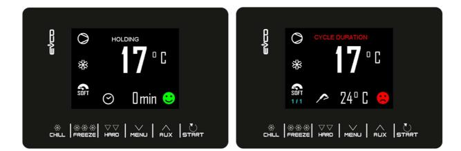
The conservation phase is not timed and is only terminated when the **STRET** key is pressed for 2 seconds. Defrosting is always enabled during a conservation phase.
