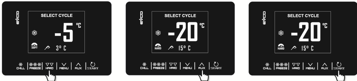
Example of a temperature controlled blast chilling cycle (needle), addition of a hard phase, quick change of the cabinet setpoint for the soft phase and start cycle.
