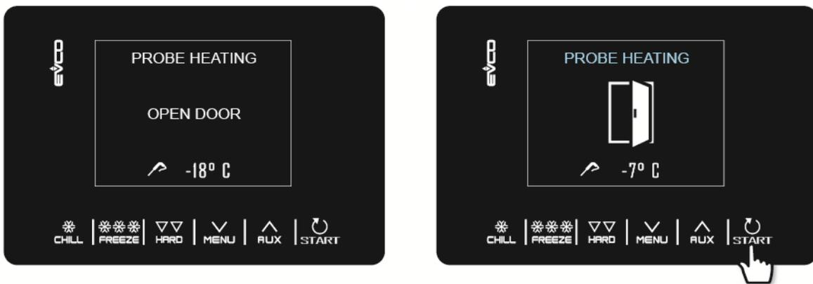
The needle probe heating output is activated at maximum for the time set by parameter u8 or until the temperature indicated by the needle probe has reached that set by parameter u7.
