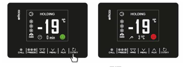
The conservation phase is not timed and is only terminated when the START key is pressed for 2 seconds.
