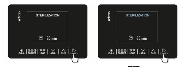
Sterilisation ends when the time set by parameter u6 has elapsed, after the **START** key has been pressed for 2 seconds or if the door is opened.
