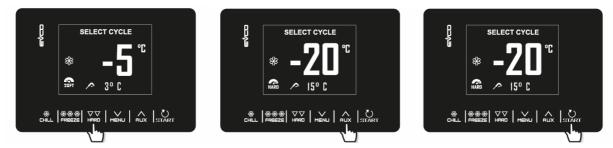
Example of a temperature controlled blast chilling cycle (needle), addition of a hard phase, quick change of the cabinet setpoint for the soft phase and start cycle.
