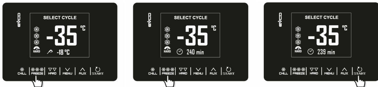
Example of a temperature controlled blast freezing cycle (needle), conversion to time controlled cycle, quick change of the blast freezing cycle duration and start cycle.
