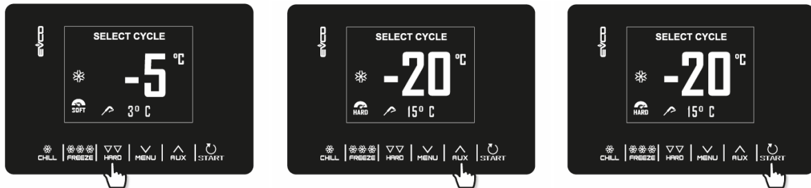
Example of a temperature controlled blast chilling cycle (needle), addition of a hard phase, quick change of the cabinet setpoint for the soft phase and start cycle.
