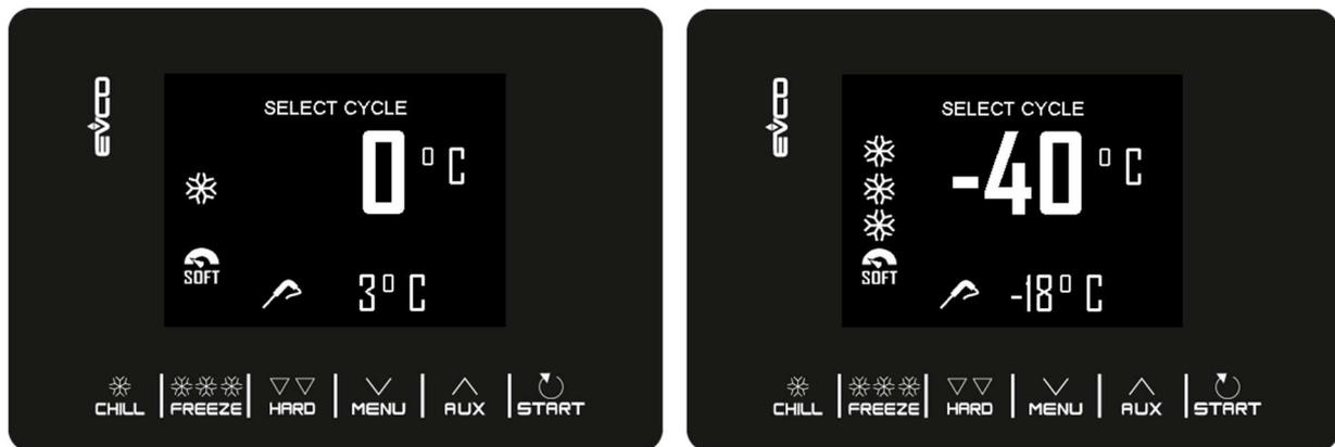
In addition to the blast chilling and blast freezing cycles, the controller is able to manage the following **special cycles**, some of which are always available, while others can be enabled/disabled by parameters u1 (load managed by the K4 output) and u2 (load managed by the K5 output):
