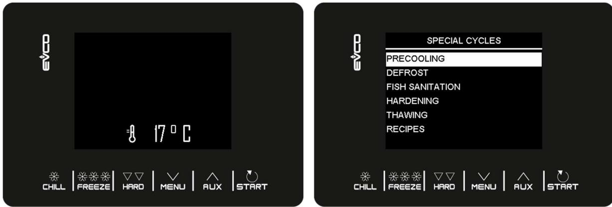
While the cycle is being carried out, the display will show the most significant data:
