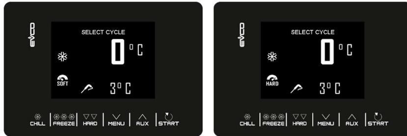
The selected cycle will offer either the pre-loaded settings for that cycle, or the settings of the last cycle carried out (depending on the r36 parameter). By pressing **AUX** **MENU**, it will be possible to quickly change the value of an individual data item (set by parameter r35) within the permitted ranges.
