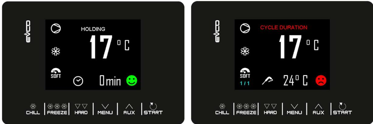
The conservation phase is not timed and is only terminated when the **START** key is pressed for 2 seconds.
