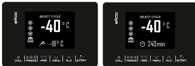
If it is a temperature controlled cycle, a test will be performed to check that the needle probe has been correctly inserted in the food item to be blast chilled. If the test is not successful, the cycle automatically switches to time controlled mode: the buzzer sounds and the type of cycle control is converted from temperature to time on the display. For more details about how to run the test, see section 6.2.
