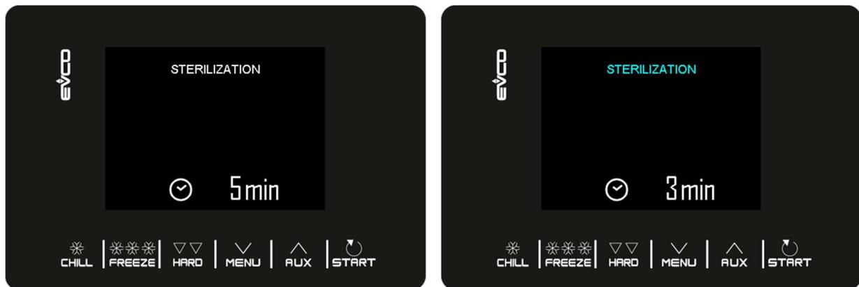
Sterilisation ends when the time set by parameter u6 has elapsed, after the **START** key has been pressed for 2 seconds or if the door is opened.
