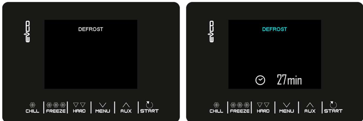
Defrosting can also be carried out automatically during conservation or pre-cooling at time intervals set by parameter d0, provided that this value is not set to 0.
