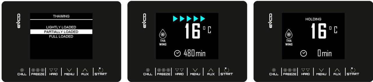
The defrosting cycle is managed on the basis of the amount of product to be defrosted that is loaded into the unit in relation to the maximum quantity specified by the manufacturer. To keep it simple, the load quantities that can be selected are divided into three bands, for each of which the controller will load three different sets of predefined parameters, in accordance with the following scheme:
