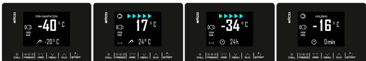
During a sanitation cycle, the device will always display the cabinet temperature and, depending on the phase in progress, the blast chilling end temperature or the duration of the holding phase.
