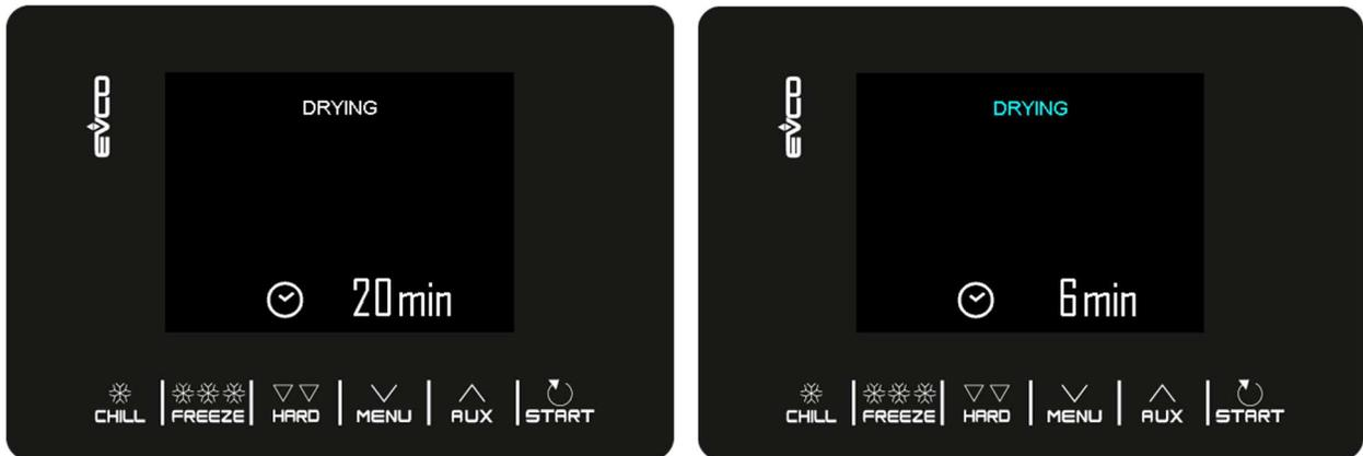
The drying cycle stops when the time set by parameter e1 elapses, when pressing the key **START** for 2 seconds or when the maximum cabinet temperature set by parameter e2 is reached. During drying the evaporator fans are active. The display will show the count-down for the remaining time. At the end of the cycle the buzzer sounds for 1 second and the device returns to the Home page
