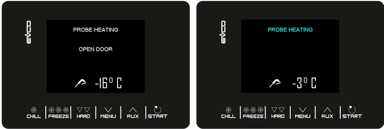
The needle probe heating output is activated at maximum for the time set by parameter u8 or until the temperature indicated by the needle probe has reached that set by parameter u7.
