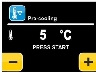
Use the + and - keys to set the desired pre-cooling set-point; use the START button to start the machine up. The cycle has infinite duration until a program is launched. When the first work set-point is reached, the controller will emit an acoustic signal
