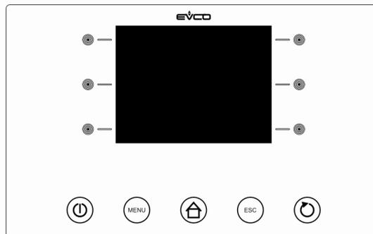
During the ON status, the device will display the date, real time, cabinet temperature and the possible functions that can be selected.
