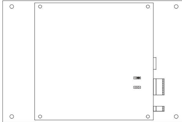
To disconnect the terminating resistors, position the jumper as illustrated in the following drawing.
