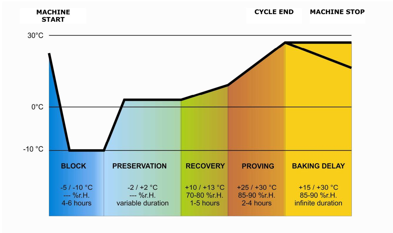
An automatic retarder-proofer cycle is composed of 5 different phases with different temperatures, relative humidity, fan speed and duration, which are performed one after the other and precisely:
