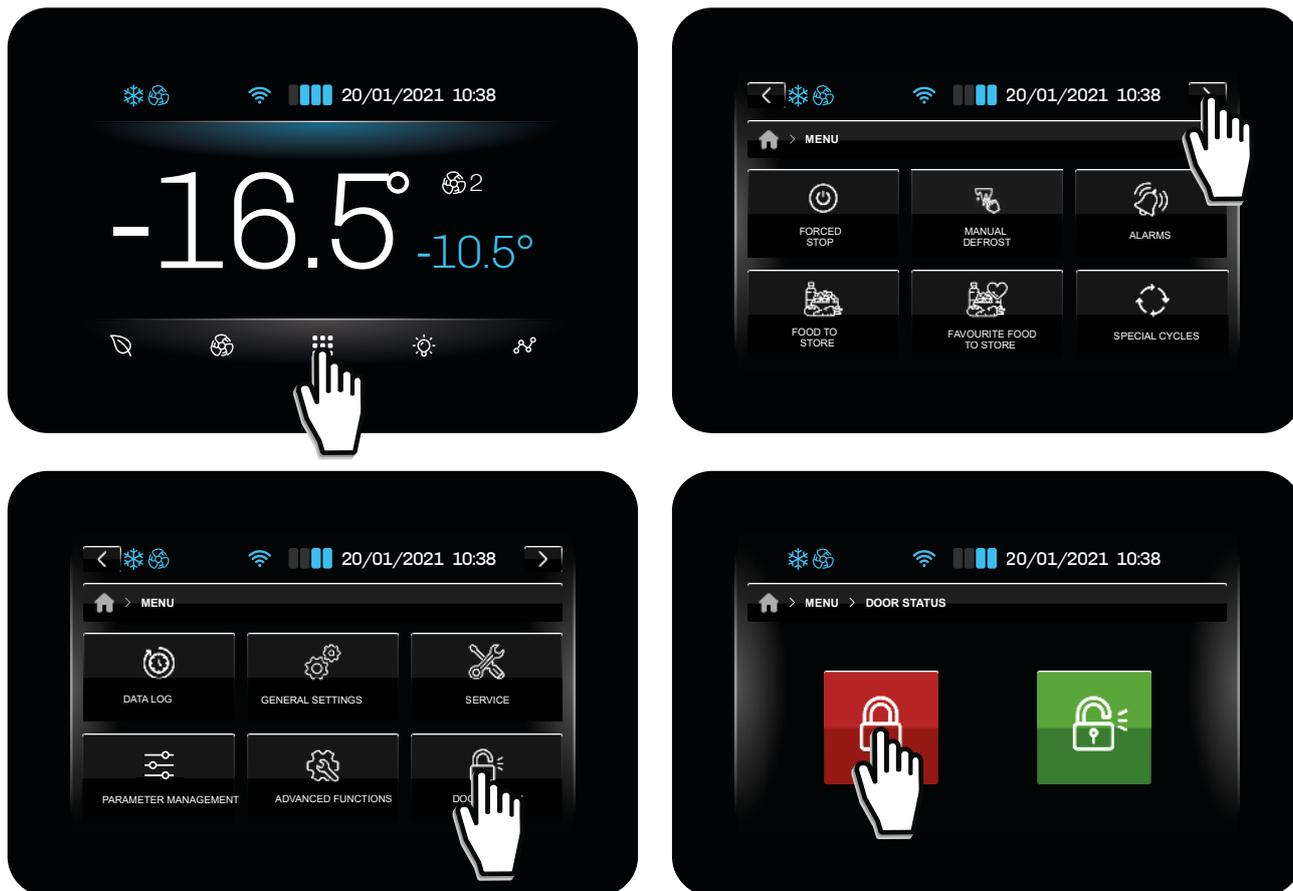
Fig. 22. Door lock/unlock
