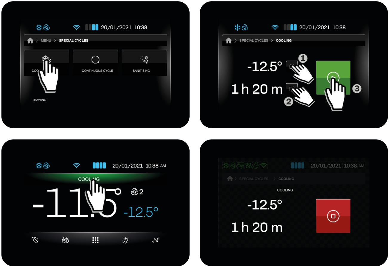
Fig. 39. Cooling cycle
