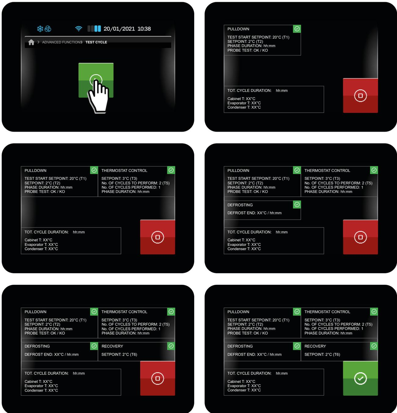
Fig. 49. Test cycle phases
