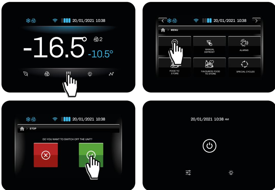
**Fig. 18.** Controller ON/OFF
