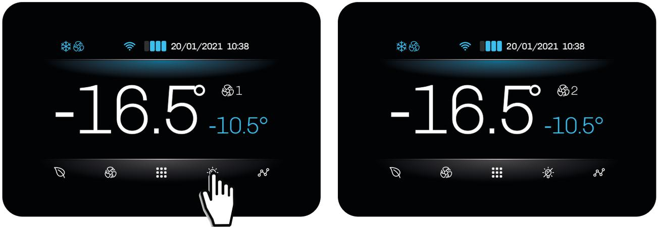
Fig. 31. Switching cabinet light on/off
