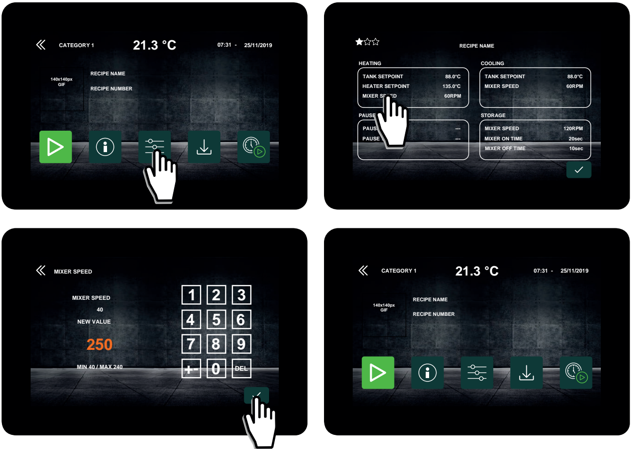
Fig. 37. Changing recipe values before the cycle starts or while it is in progress
