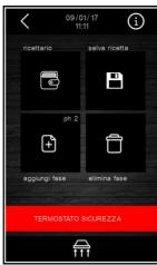
If no cooking cycle is in progress, the following functions can be activated.  $\label{eq:cooking}$
