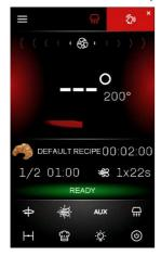
Pressing the alarm icon will silence the buzzer and the page with the active alarms will automatically be displayed.
