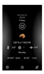
Briefly press the ON/OFF key to switch the device on.
