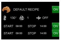
ON will start up pre-heating of the set recipe, according to machine configuration.
