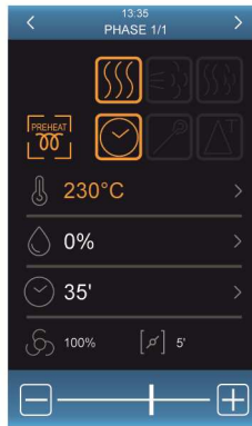
Setting the working setpoint.
