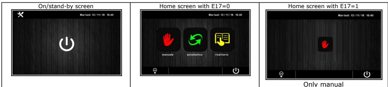
To switch the device on, press the central key on the On/stand-by screen; to switch the device off, press the key on the lower part of the Home screen.
