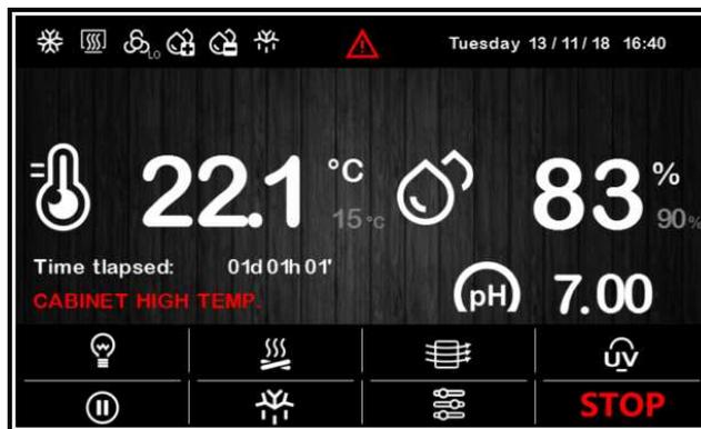
The top bar indicates the status of the main regulation outputs/status (hot / cold / humidification / dehumidification / ventilation / defrosting status), any alarm in progress (an alarm icon is always given with the description) and the current time-date.
