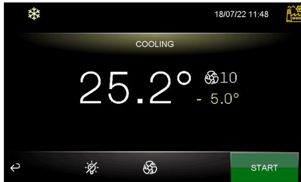
The values of the temperature setpoint and fan speed can be changed before starting up the desired cycle; if a timer is not set to end the cycle after the pre-determined time, the cycle will continue indefinitely. To enable a timer, set parameter E11 to 1. The time is set by parameter MC4. Pressing the **INF key** (infinite time) on the bottom right of the display, the time is disabled for that cycle. Once the cycle is deselected, the value of MC4 is restored.
