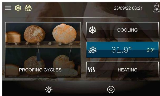
When it reaches the temperature setpoint for the first time, the buzzer will sound. If the temperature in the cabinet is equal to or lower than the setpoint, the pre-cooling function cannot be activated. The pre-cooling function is of infinite duration and ends as soon as a retarding-proofing, cooling or heating cycle is started up. To manually terminate the pre-cooling cycle, press the blue key showing the temperature.
