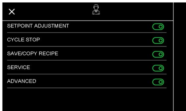
Once the user configurations have been completed, it is possible to log out manually from the Home page by pressing the icon of the user who is currently active, otherwise the controller will exit after 5 minutes.
