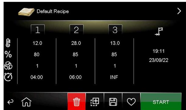
The image or description of the recipe can be set or changed in this screen; touch the image on the recipe (at the top left) and a library of images loaded by the manufacturer will open:
