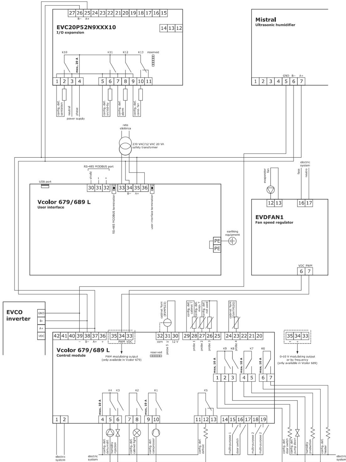
\*The USB communications port makes it possible to upload and download the device settings and personalise the graphics, recipes and languages using an ordinary USB flash drive (see section 11 "USB PORT MANAGEMENT").
