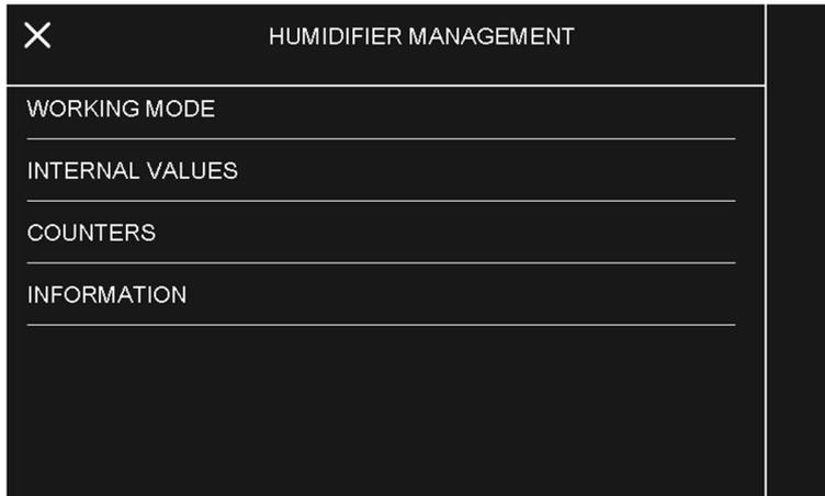
WORKING MODE: this page gives the internal working values of the humidifier and can also be viewed while a cycle is running by pressing the function key
